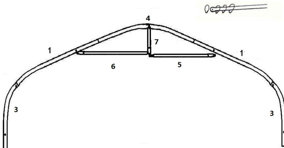
3. On each end of (no.1), install the Leg (no.3). Repeat step 1 for all frames.
