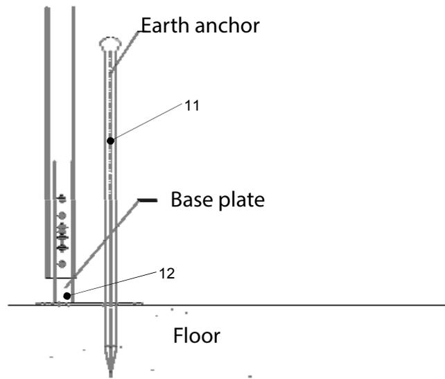
6.) Take the pagoda in position. After this fix the side-covers. Hit the earth-anchors (11) into the available holes of the base-plate (12). Each pagoda, comes with 4 earth-anchors.
