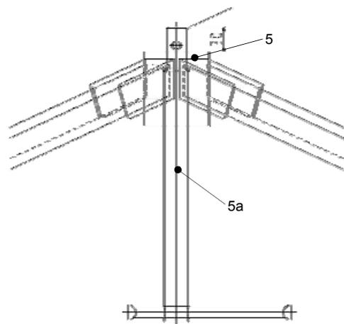
3.) Take the ridge-piece (5) and turn the spindle (5a) down until the top comes out 3 cm. Lift the beams (4) to fit them in the ridge connectors, smoothly.
