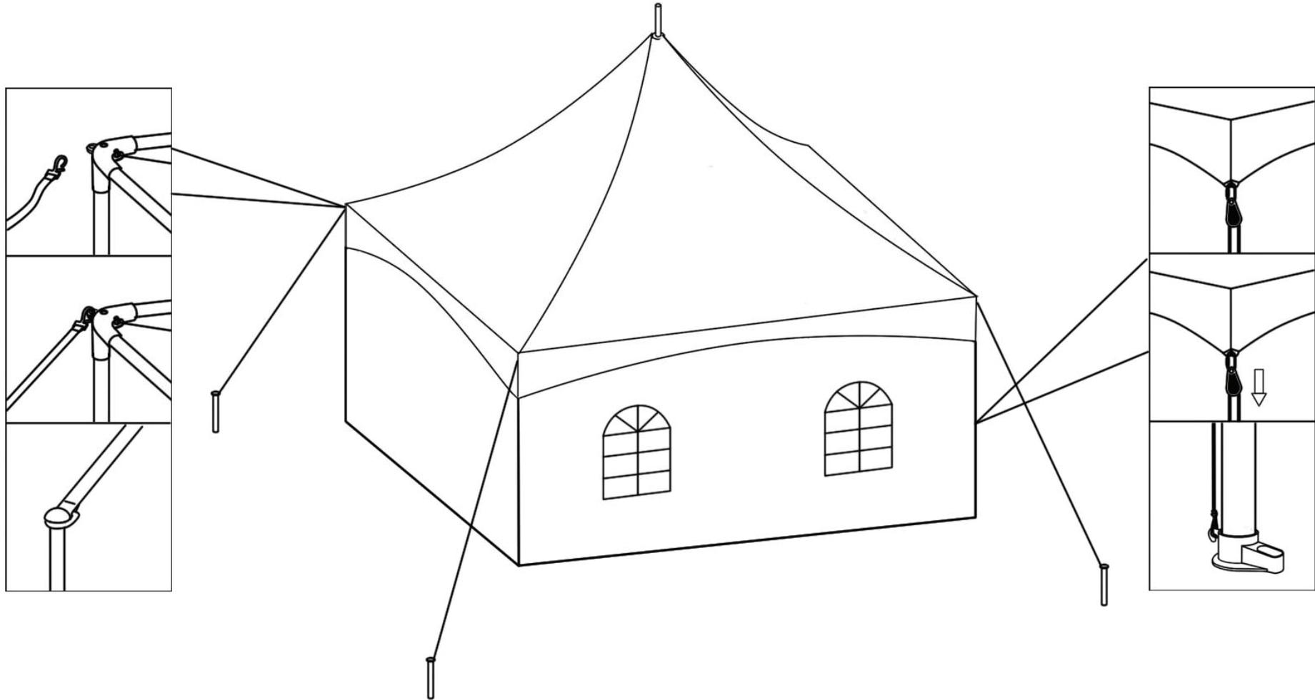
**Step 9:** Fasten the roof tensioning ropes and use the roof tensioning straps make the tent more stable.
