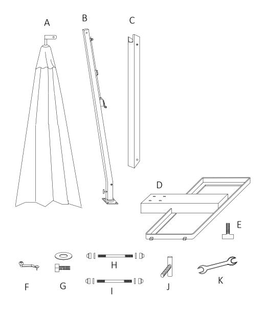
Step 1: Fixing the 8 feet (E) into the base's metal frame (D), try to find a flat ground to put it on.
