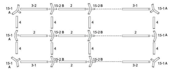
To ensure the screw fixed to every pole tightly. And then use the turnbuckle and steel tension bar to tighten the top structure.
