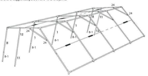
Attach the another supported poles (1.8.8-1) to the joints, built-up the framework.
