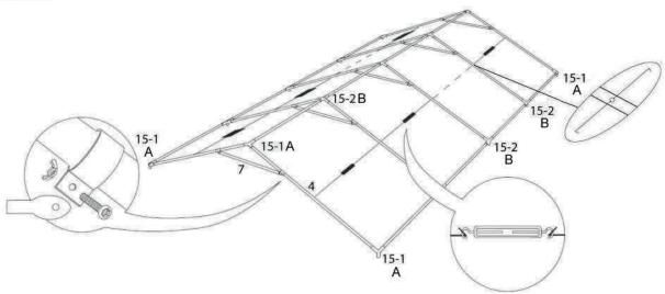
Attach one end of supported pole (1.8.8-1) to the joints
