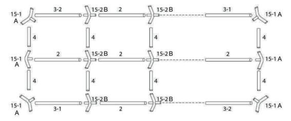
To ensure the screw fixed to every pole tightly. And then use the turnbuckle and steel tension bar to tighten the top structure.
