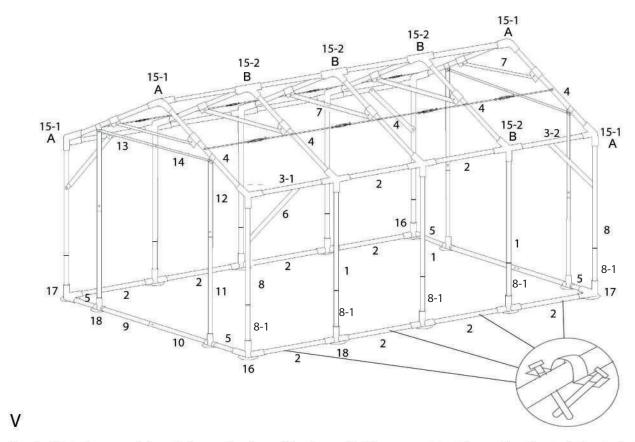
You facilitate the assembly and dismantling by pulling the roof with ropes ont tent frame. Use the steel clips to fasten the cover to the frame. Each section we offer bracket and nail to fasten the frame to ground.
