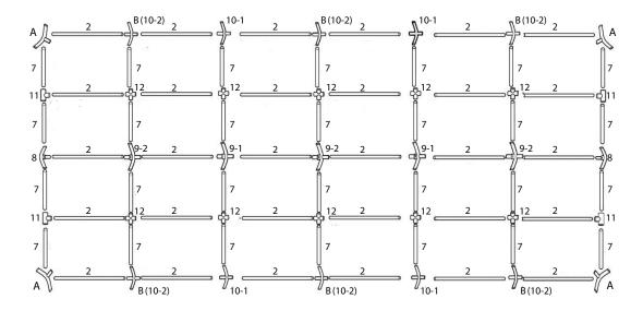
Attach one end of supported pole (4.5) to the joints (8. 11. 9-1. 9-2. 12)
