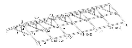
Fastening the roof by using turnbuckle set (25) which are diagonally across through each two sections as shown below.
