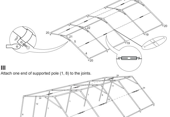
Attach the other supported poles (1, 8) to the joints, built-up the framework.
