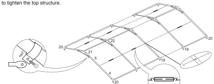
Attach one end of supported pole (1, 8, 8-1) to the joints.
