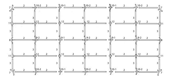
Attach one end of supported pole (4.5) to the joints (8.11.9.12)
