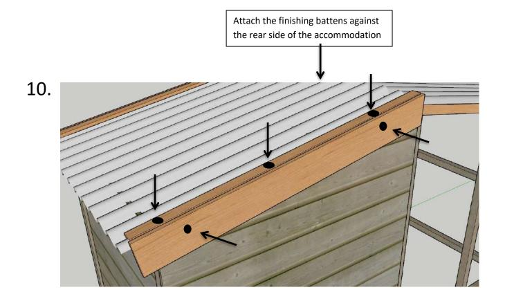
Screw the batten against the rear side of the accommodation
