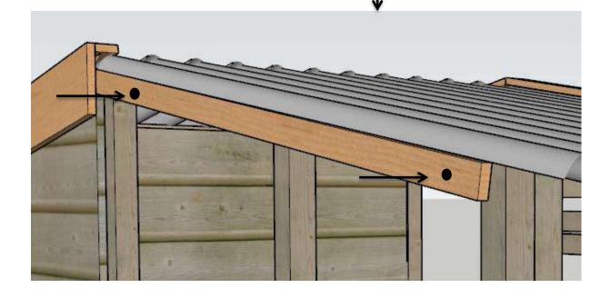
Screw the right finishing lath in the same way as the left finishing lath
