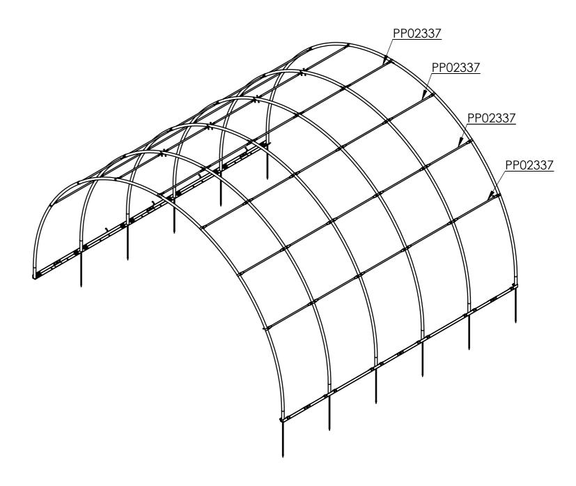
mounting instruction - mounting of struts for section
