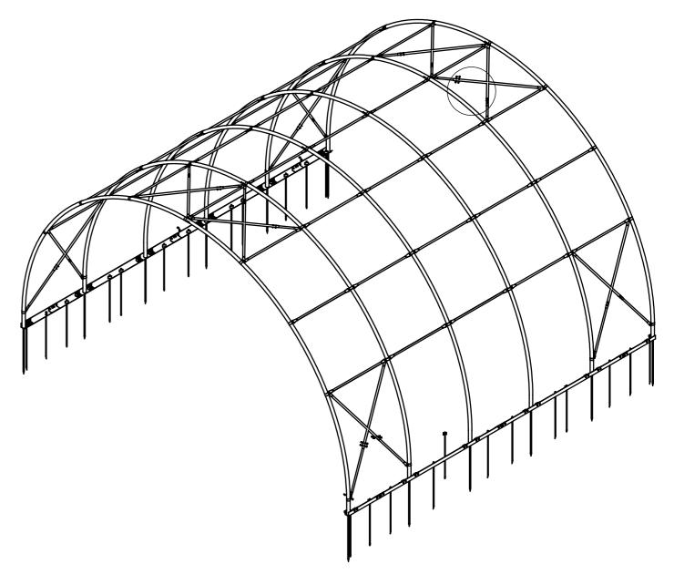
note: extra struts used in first section and in the hall from 15m length
