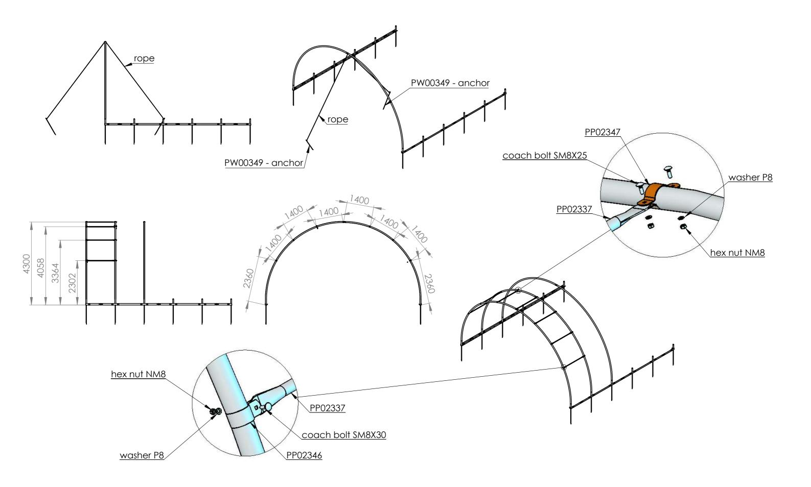
mounting instruction - mounting of struts for section
