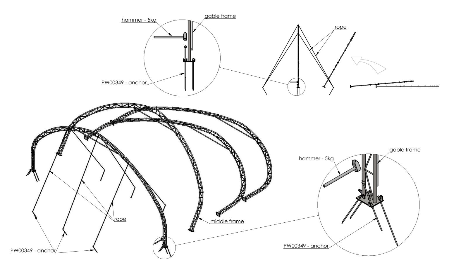
mounting instruction - mounting of struts for first section
