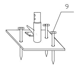
Figure 3 As Figure 3 shows, each base flange is equipped with three stake pegs.
