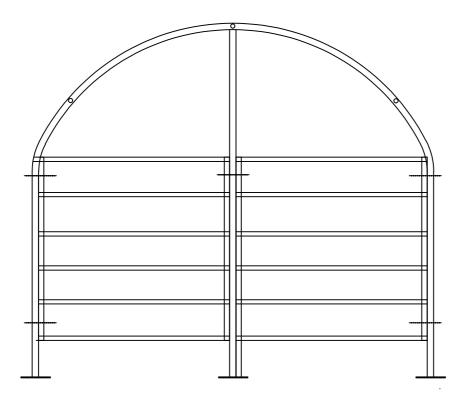
Figure 12 Fastening the two ends of the Roof Cover
