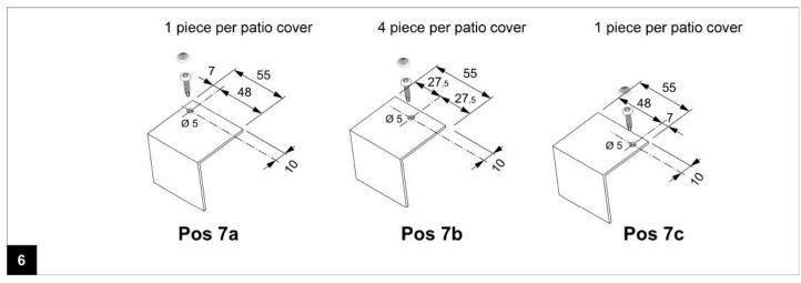
Drill the Angle Plates as shown in above Details
