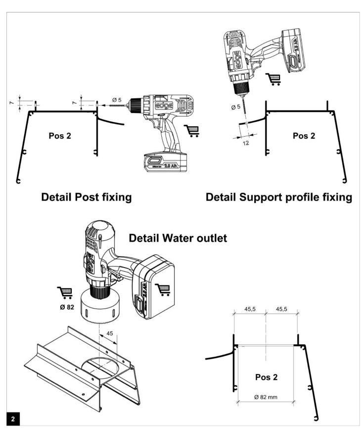
Drill the Gutter profiles according to the above Details and dimensions shown in step 1
