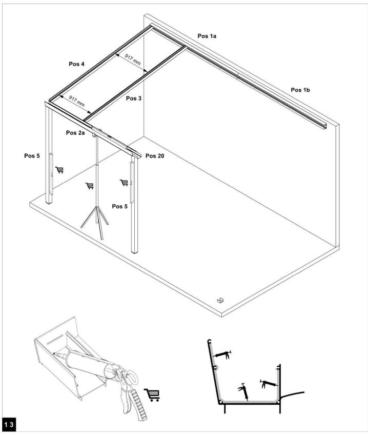
Assemble the first intermediate support (cut to size), check again to ensure everything is still straight, square and level! Thoroughly seal the Gutter and End plate connection to ensure it is watertight!
