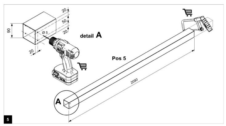
Drill the Post according to the above Detail and Dimensions and cut them to size if mounting on the floor! When mounting the Posts in the ground, do not shorten posts!!
