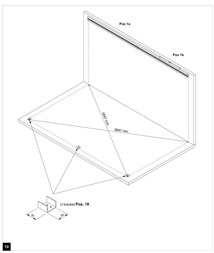
Mount the 2nd part of the Wall profile level on the wall! Check the squareness of the patio cover with the diagonal measurements!
