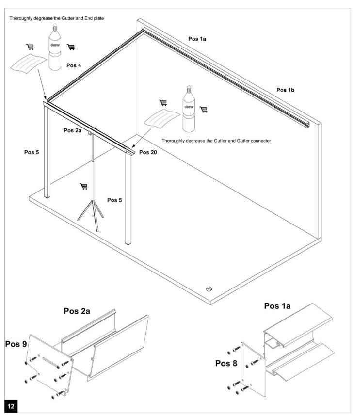
Assemble the first part of the Gutter and assemble the first Side support!
