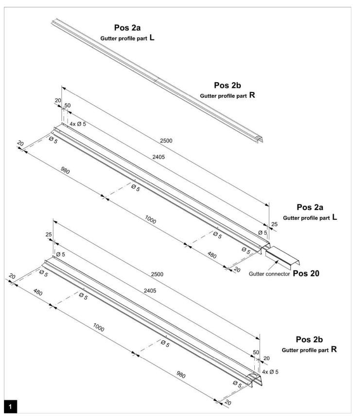
Drill the Gutter profiles according to the above dimensions and Details shown in step 2
