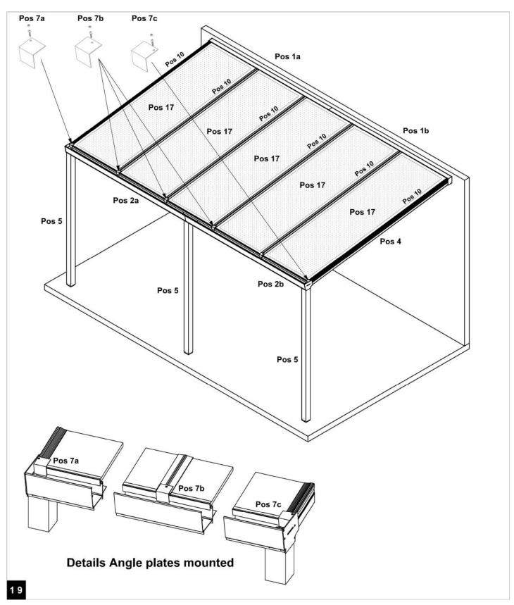
Fix the Angle plates with 4.2x32 screws! Place the supplied screw covers on all screws!
