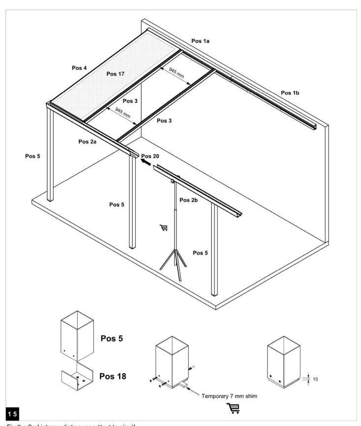
Fix the 2nd intermediate support(cut to size)!
