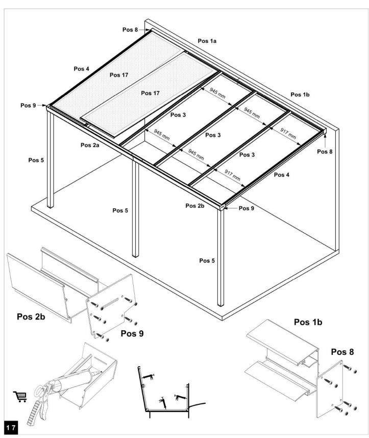
Assemble the remaining intermediate Supports according to the setting out shown above! Mount the End plates to the right end of the Gutter and the Wall profiles!
