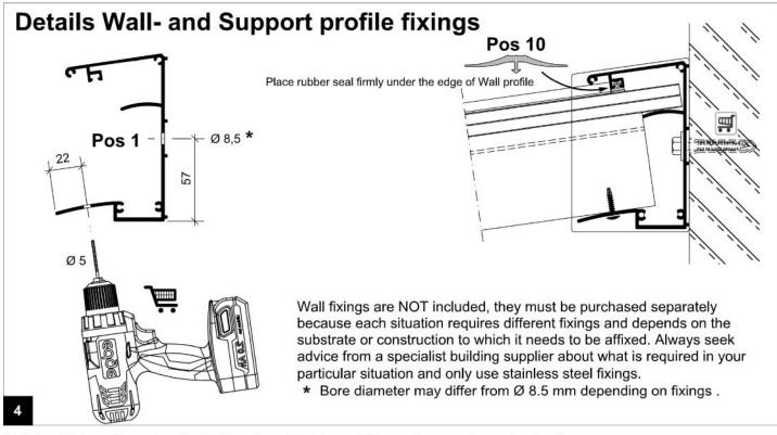
Drill the Wall profiles according to the above Details and Dimensions as shown in step 3
