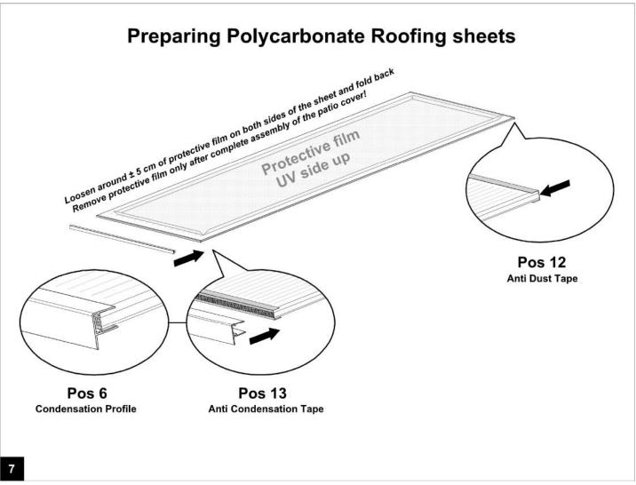
Stick Anti Dust Tape over the end of the Polycarbonate which is at the top of the patio cover!
