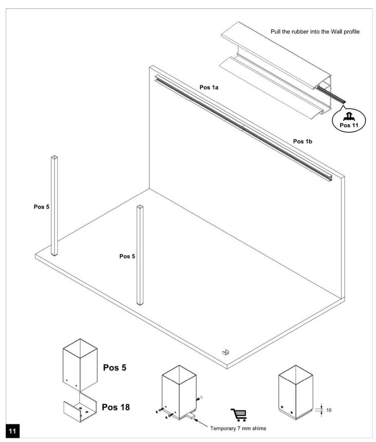
Slide the first 2 posts over the U brackets and keep them 10 mm from the floor due to drainage! Use 7 mm shims to temporarily keep the posts up and screw the posts to the U brackets! Pull the Rubber into the Wall profile!
