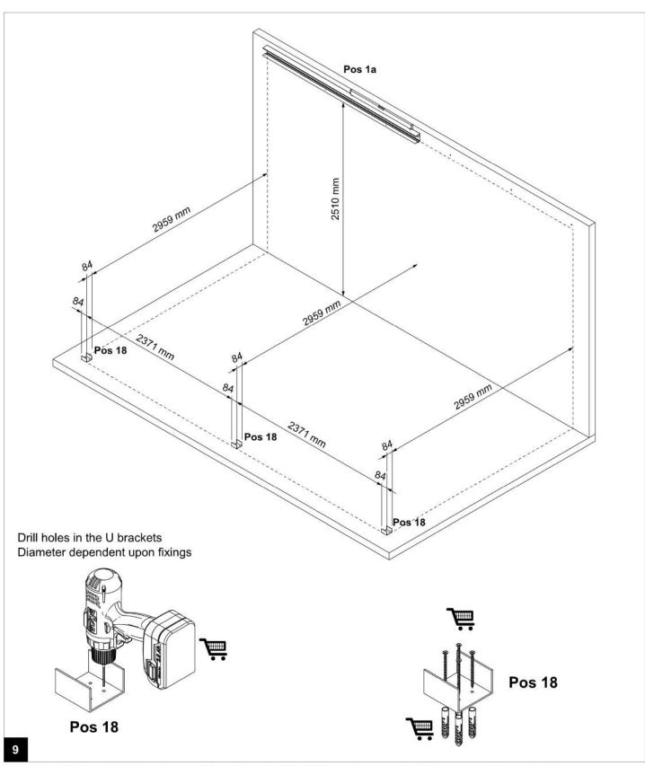
Attach the U-elements to the floor and the 1st part of the Wall profile according to the above dimensions! Floor and wall fixings are NOT included, they must be purchased separately because each situation requires different fixings and depends on the substrate or construction to which it needs to be affixed. Always seek advice from a specialist building supplier about what is required in your particular situation and only use stainless steel fixings!
