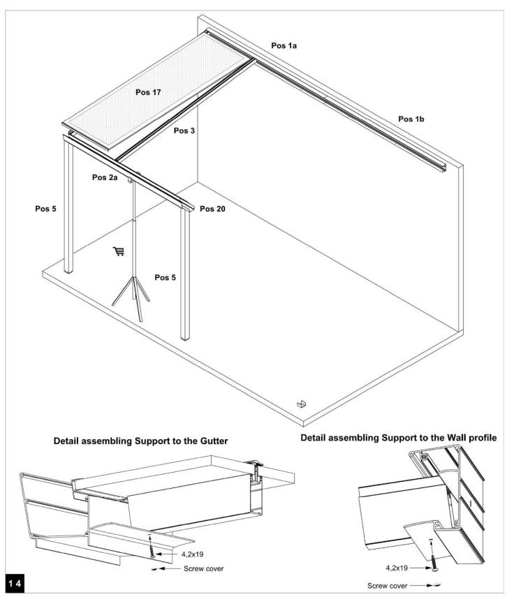
Advice: Place the first Polycarbonate sheet in the first section, this sheet ensures that the roof surface stays square!
