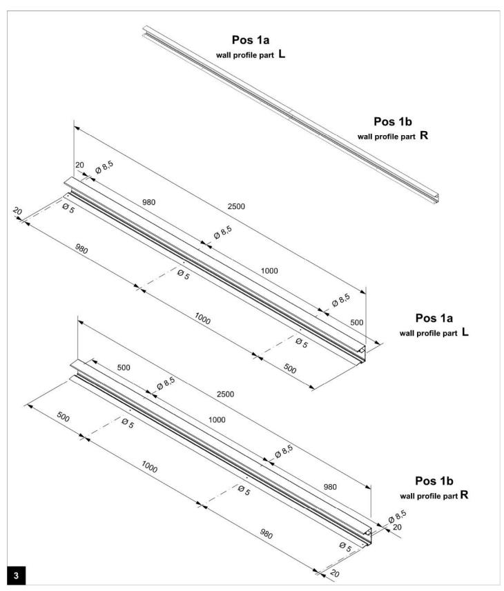
Drill the Wall profiles according to the above dimensions and Details shown in step 4
