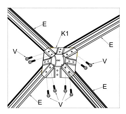
STEP 6:Assemble the Roof Frame by Attaching the Roof Ribs Long (Part E) to the Roof Top Brace (Part K1).
