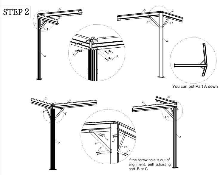
STEP 2:Attach Crossbeams 1 (Part B) and Crossbeams 4 (Part C) to Pillars (Part A). Attach Support Brackets (Parts F and F1) to Crossbeam and Pillar. Attach Crossbeams 2 (Part C) and Crossbeams 3 (Part B) to Pillars (Part A). Attach Support Brackets (Parts F and F1) to Cross Beam and Pillar.
