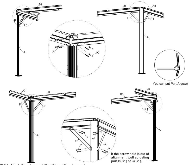
STEP 2: Attach Crossbeams 1 (Part B) and Crossbeams 4 (Part C1) to Pillars (Part A). Attach Support Brackets (Part F and F1) to Crossbeam and Pillar. Attach Crossbeams 2 Part B1) and Crossbeams 3 (Part C) to Pillars (Part A). Attach Support Brackets (Parts F and F1) to Cross Beam and Pillar
