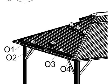
Note: First fix 4 (Part M2) with V, but do not screw too tight, then install (Part G1 G2 G3 and G4 )as shown in the diagram. You'd better from left to right. Attach the Center Rib Braces (PartM1) as shown in the diagram.
