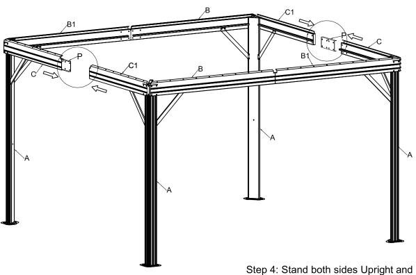
Step 4: Stand both sides Upright and Connect Crossbeams B and Crossbeams B1 using the Crossbeam Connectors (Part P).
