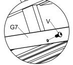
Gently insert Z2, Z3, Z4 from left to right as shown, then tighten them via screws U1 and V.
