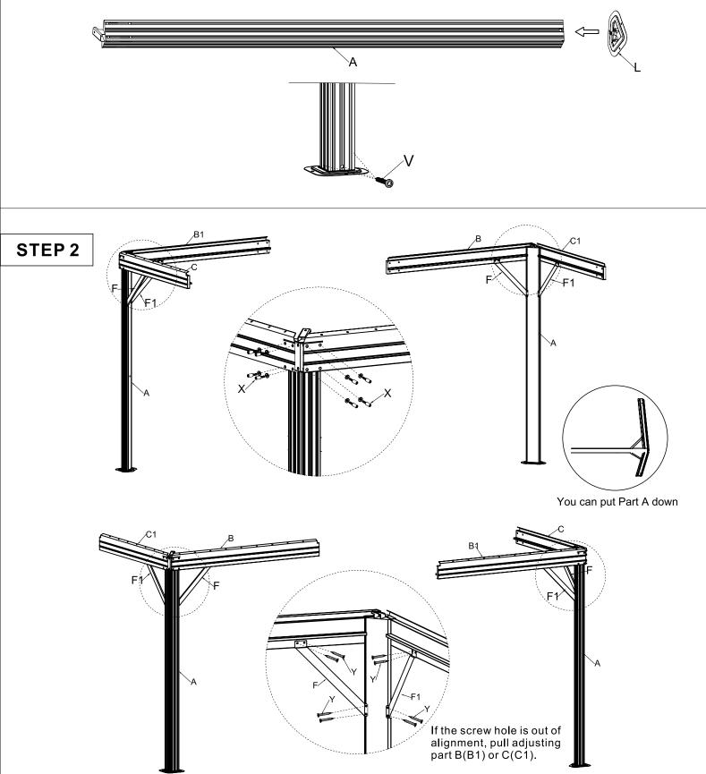
STEP 2: Attach Crossbeams 1 (Part B) and Crossbeams 4 (Part C1) to Pillars (Part A). Attach Support Brackets (Parts F and F1) to Crossbeam and Pillar. Attach Crossbeams 2 (Part B1) and Crossbeams 3 (Part C) to Pillars (Part A). Attach Support Brackets (Parts F and F1) to Cross Beam and Pillar.
