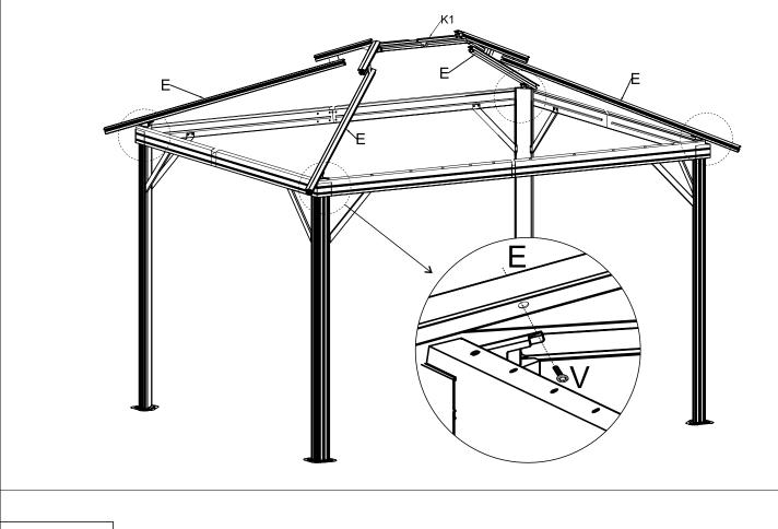
STEP 7: Lift the Partially assembled Roof on to the assembled Frame and attach.
