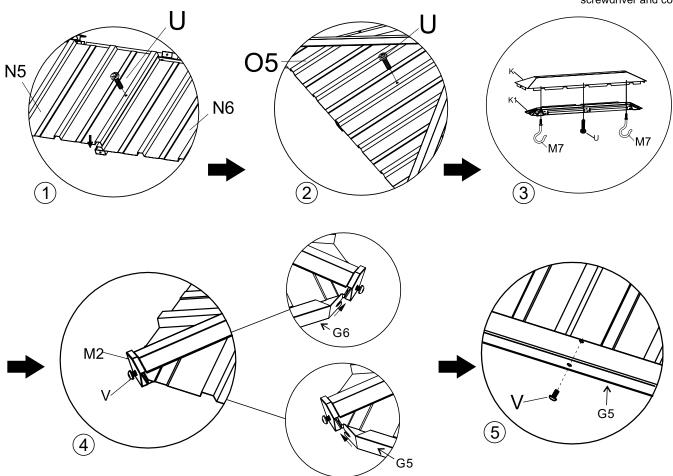
Step11-2: First fix 4 (Part M2) with V, but do not screw too tight, then install (Part G5 and G6) from left to right.
