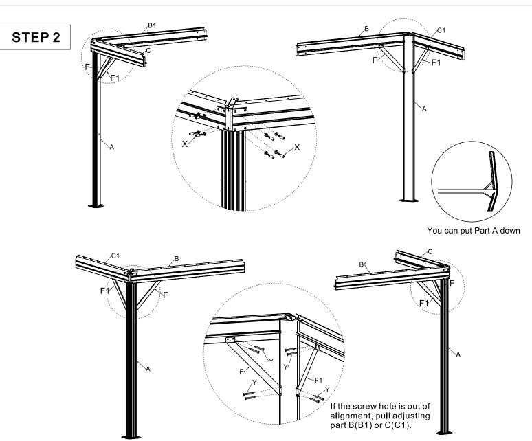
STEP 2: Attach Crossbeams 1 (Part B) and Crossbeams 4 (Part C1) to Pillars (Part A). Attach Support Brackets (Parts F and F1) to Crossbeam and Pillar. Attach Crossbeams 2 (Part B1) and Crossbeams 3 (Part C) to Pillars (Part A). Attach Support Brackets (Parts F and F1) to Cross Beam and Pillar.
