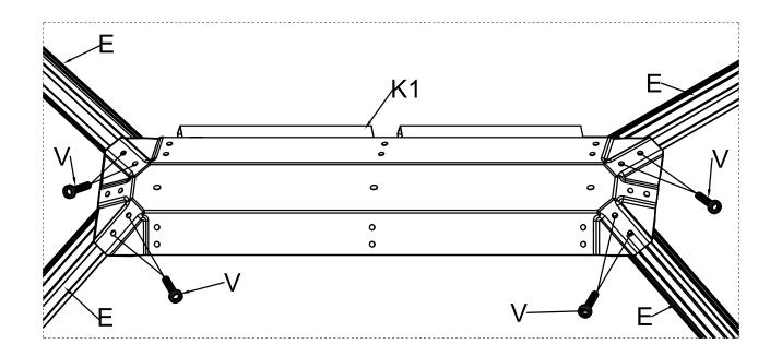
STEP 6: Assemble the Roof Frame by Attaching the Roof Ribs Long (Part E) to the Roof Top Brace (Part K1).
