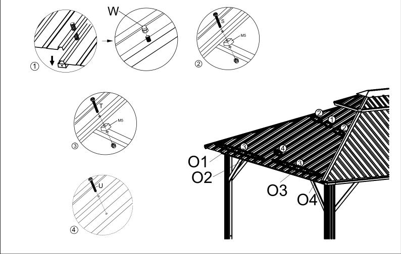
Note: First fix 4 (Part M2) with V, but do not screw too tight, then install (Part G1 G2 G3 and G4 )as shown in the diagram. You'd better from left to right. Attach the Center Rib Braces (PartM1) as shown in the diagram.
