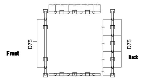
First lay out the cills, connectors and anchor brackets approximately in place, then tighten them with bolts and nuts which provided.
