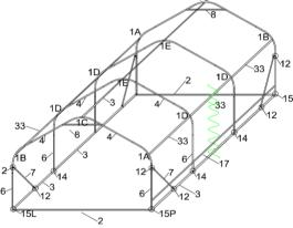
2 Assembly of the front and back wall with door
