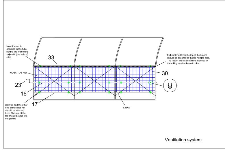
The "Main part of the tunnel" piece is extra long on both sides. The extra cover must be dug into the ground to secure the polytunnel greenhouse.
