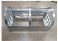
**14.** Seal the edges of the polycarbonate with the added aluminum strip (13).
