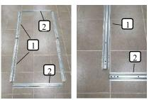
2. Join the corner parts of the structure (1; 2) with the corners for connecting the rear and side parts (5). Use M5x16 mm bolts (9) with nuts (11). Do the same for all 4 corners.
