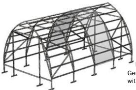
**Fig. 1a** ONE "INSERT" extends the greenhouse by 2.13 m. Number of the inserts for the greenhouse is not limited
