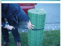
When the roll is complete, stand it on its end with the tongue side on top. Place a roll strap around the roll to keep it from coming undone.
