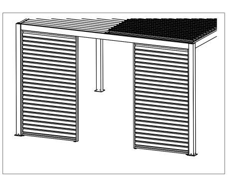
STEP9: Note that the hole on the upper beam fixing part is towards the inner side of the pergola
