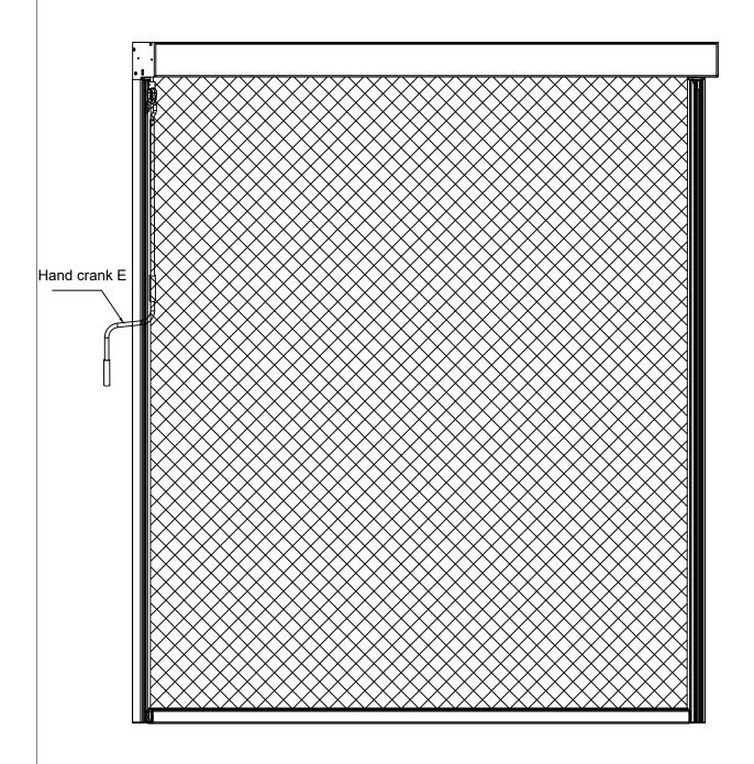
After installing the plastic fabric clamping profile B3 place the fabric completely down in order to adjust the fabric. Then install the insertion rail as described below.
