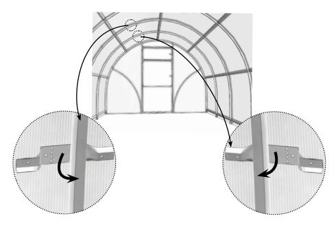
Fasten the clamps to the arches using self-tapping screws. Install **C.02** purlin in the clamps.
