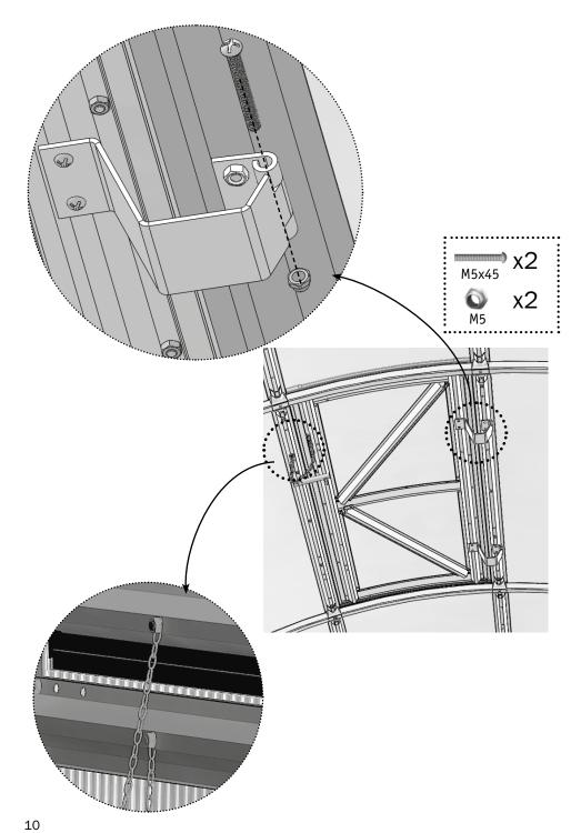
The window security chain is fastened with screws and keeps the vent during the gusts of wind.
