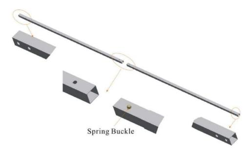
2. Press the spring buckle and then put this tube into the other tube until the spring buckle is locked; see the picture below:
